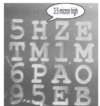
Top: An example of an engraved data matrix with a black background to make it more visible. Bottom: Engraved alphanumeric code
